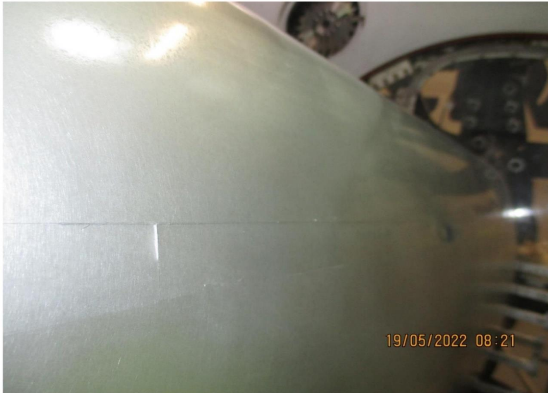
Figure 21: Chamfering on DTU-C21 suction side (down-wind).
