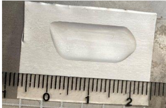
Figure 9: Plasma treated riblets which show a clear direction wetting with distinct borders.
