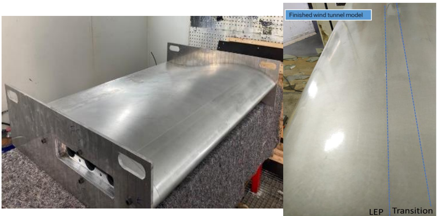
Figure 17: Finished wind tunnel model (left & right) and close-up indication where the LEP is applied (right).
