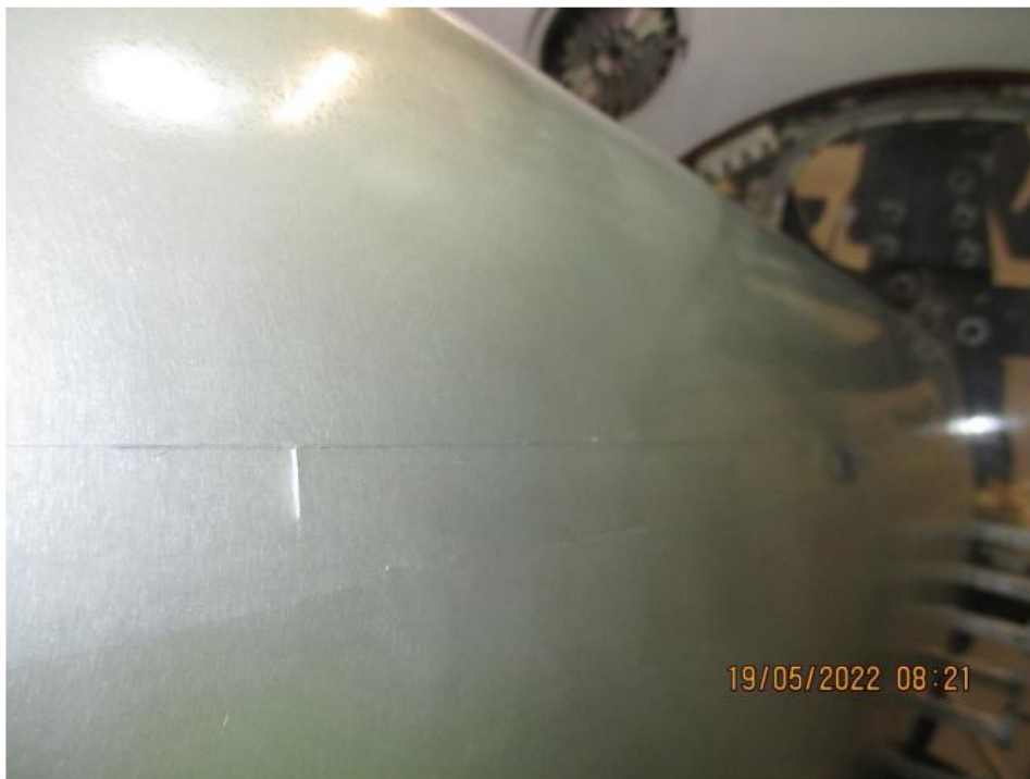
Figure 2-4: Chamfering on DTU-C21 suction side (down-wind)
