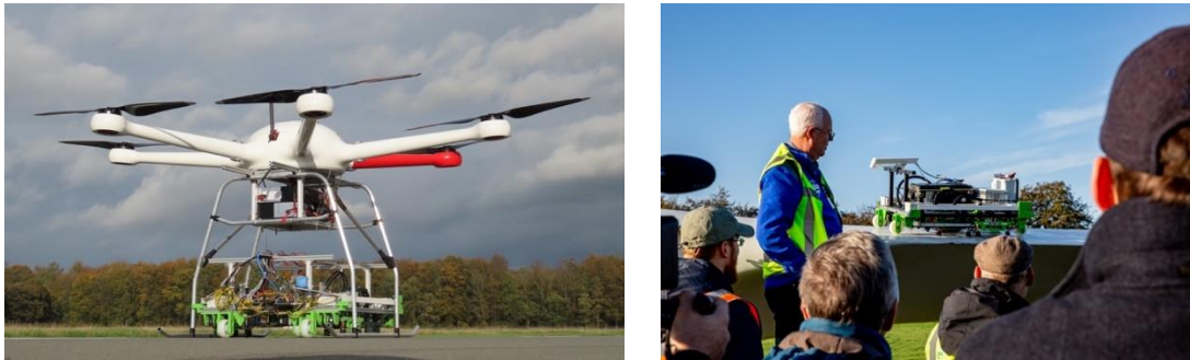
Fig.11. Drone with crawler on landing platform and crawler/sensor package on 22m wind turbine blade
