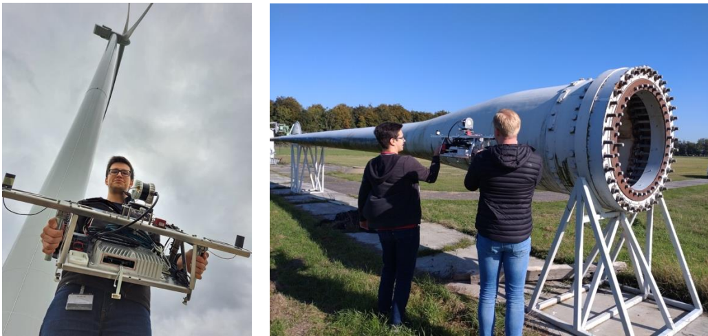
Fig.3. Lidar sensor for navigation path planning purposes (Demcon Unmanned Systems)
