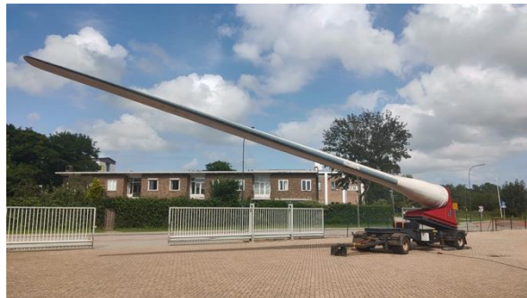
Fig.9. Mobile platform with rotatable/pitchable 22m blade
