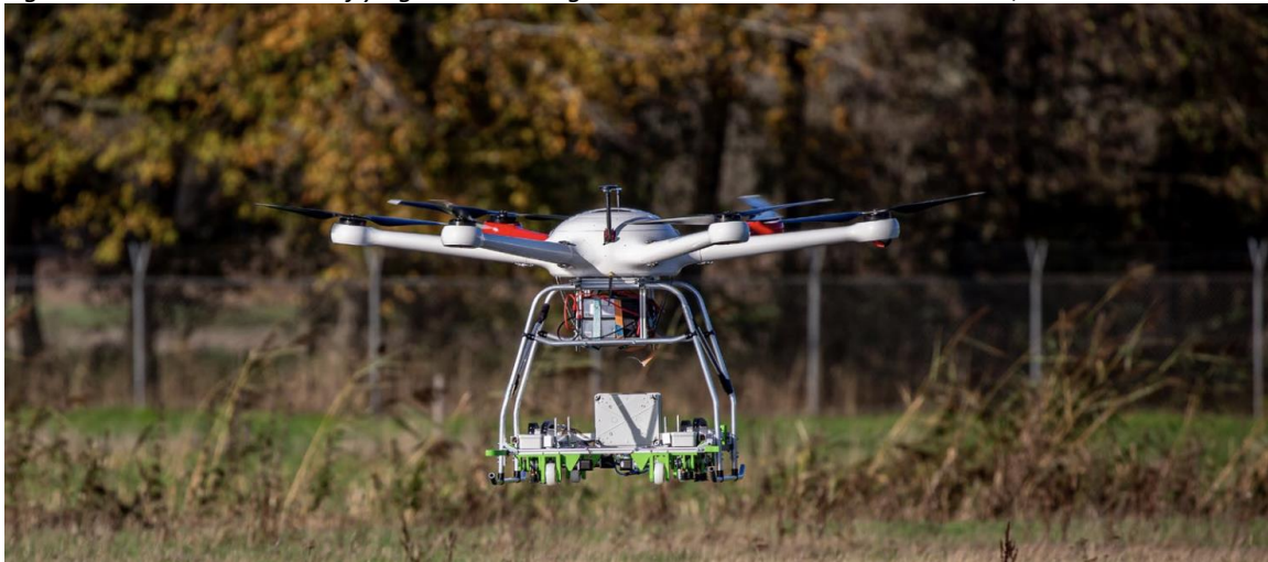
Figure 7. Drone with crawler flying at NLR during the demonstration on November 24, 2022.
