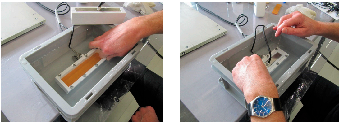
Figure 5-3: Assembly of the PAUT sliding probe under water to ensure no air is entrapped
