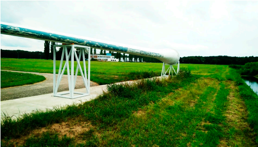
Figure 2-3: Full-scale wind turbine blade for drone experiments
