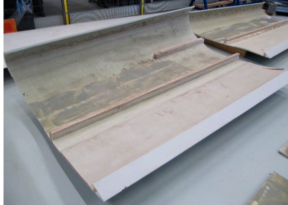
Figure 2-6: Two "full-scale" reference parts of ~2x1.70m (one bottom side, one top side)
