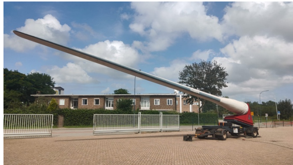
Fig.11. Mobile platform with rotatable/pitchable 22m blade
