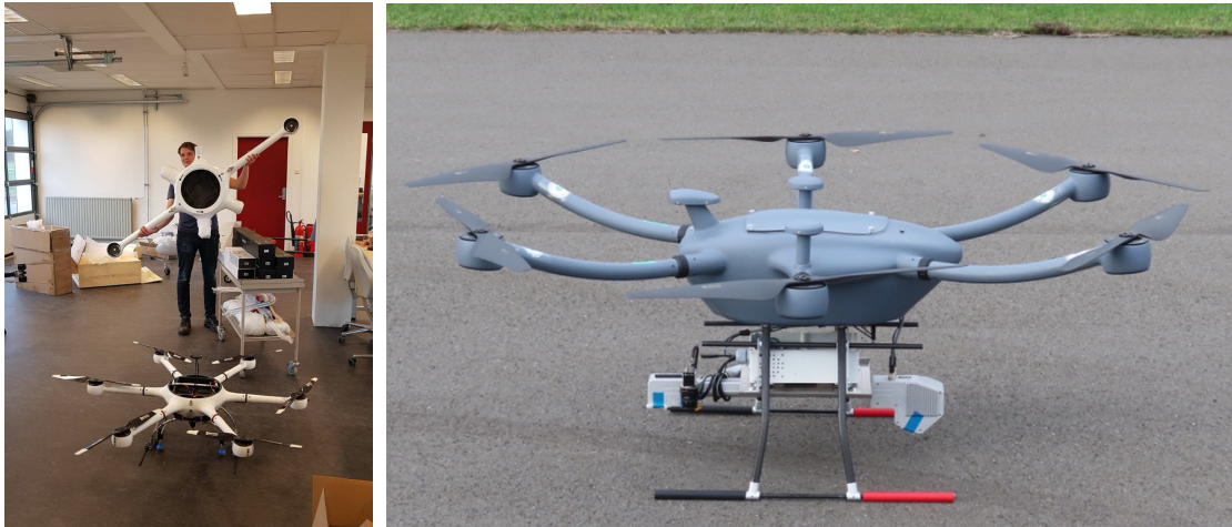
Fig.6. AIRTuB and testbed drone with laser line scanner (leading edge erosion damage TU Delft) (drones: NLR)
