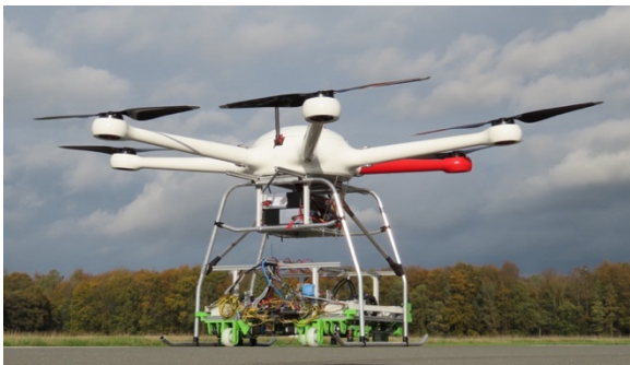
Fig.14. Drone with crawler on landing platform and crawler/sensor package on 22m wind turbine blade
